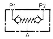
THIS VALVE HAS A 2-PIECE SPRING LOADED SHUTTLE TO PREVENT OIL FLOWING FROM PORT A' TO ANY OF P' PORTS.
