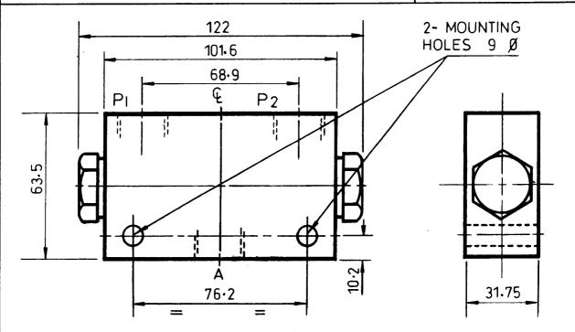
THIS VALVE IS USED WHERE A SERVICE FEED LINE HAS ALTERNATIVE MEANS OF SUPPLY, BUT ONLY ONE SUPPLY IS USED AT A TIME.
